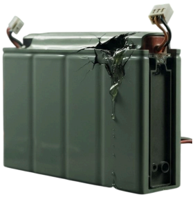
Cracked or Damaged rechargeable battery
